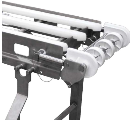
Fig. 42.31 Conveyor frames should have an open structure without horizontal surfaces and with a minimum of hidden areas/surfaces. At the outside, the framework consists of vertical plate members positioned longitudinally, which also serve as a lateral belt guide. The conveyor-frame is an all welded construction with solid round cross-members, welded at the outside frame work. The use of bolts and nuts for fastenings is reduced to a minimum. The cross-members not only act as structural frame members, but also as belt supports. The weld-on flat cross-members are provided with gaps to accommodate the freely located plastic wear strips that help to support the conveyor belt. No bolt holes or nuts were used for fastening ultra-high-molecular-weight (UHMW) polyethylene wear strips. To minimize cleaning time, these belt supports are easily lifted out of the frame by means of a quick tension-release arrangement and without manual tools. The cut-outs in the frame allow spraying and cleaning of the inside of the conveyor without lifting the belt. Although the conveyor shown is provided with a swivel-mounted roller that permits to release tension, providing improved access to the space between belt and bearing table for cleaning and disinfection. The frame member closest to the point where the belt runs onto the drive roller sprocket also serves as a guard. Stand-off legs keep fasteners out of the food zone (courtesy of Dornier conveyors).
