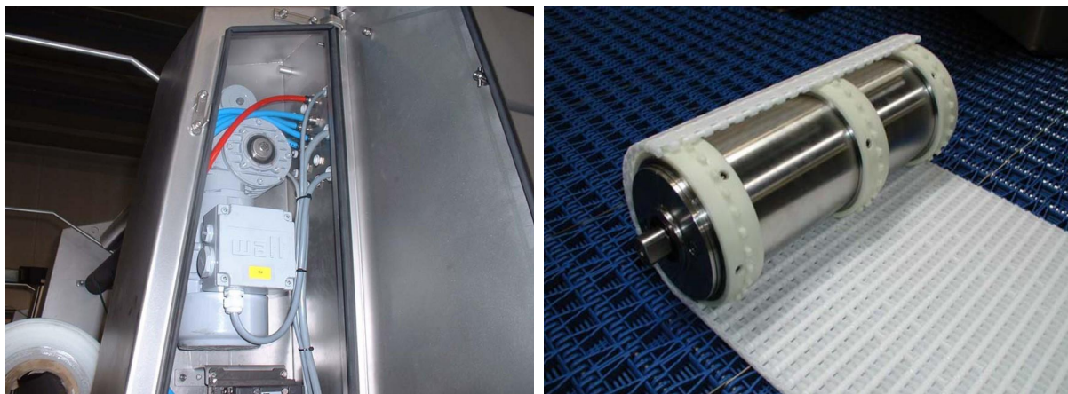
Fig. 42.33 Motors should be rather located below the line of the product flow. Both gears, chains and motors of belt drives must be covered to avoid any contamination of product. However, a chain guard (essential from an occupational safety point of view), when open, may provide a place where product may accumulate, allowing microbes to multiply to large numbers and so posing a contamination risk for the food product on the belt (courtesy of Dorner conveyors).
