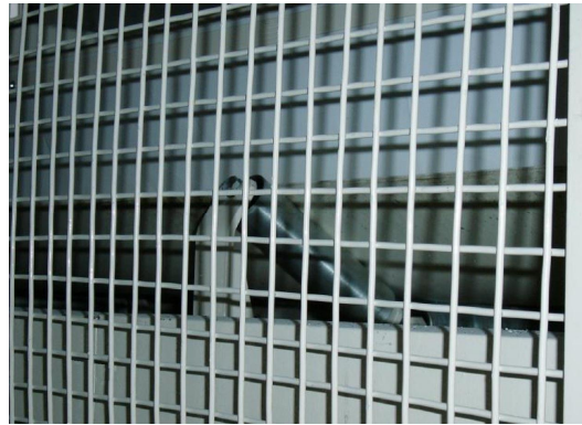
Fig. 42.37 Example of a hygienically designed guard (courtesy of P.T. Group)
