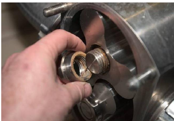
Fig. 42.49 (a) Ingress and retention of product and/or microorganisms in the threads of the rotor retaining nuts should be avoided by making use of crevice-free domed retainer nuts and by application of O-rings. (b) In a more improved version, the rotors and shaft should be designed as an integral construction. With the ports arranged in the vertical plane, it is possible to drain the lobe pump casing (courtesy of Burggraaf & Partners and Johnson Pump)
