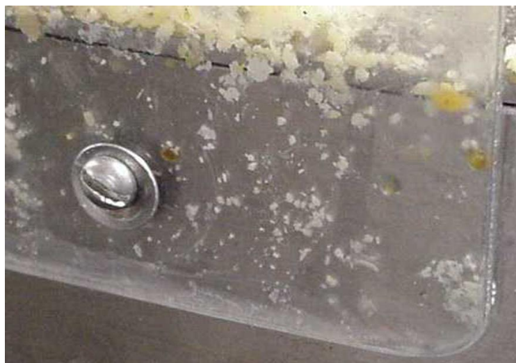
Fig. 42.3 Product contact surfaces of this equipment are not readily accessible for manual cleaning and disinfection. Moreover, the dome screw with drive slot and washer create gaps and crevices where debris collects (courtesy of Joe Stout, American Meat Institute).
