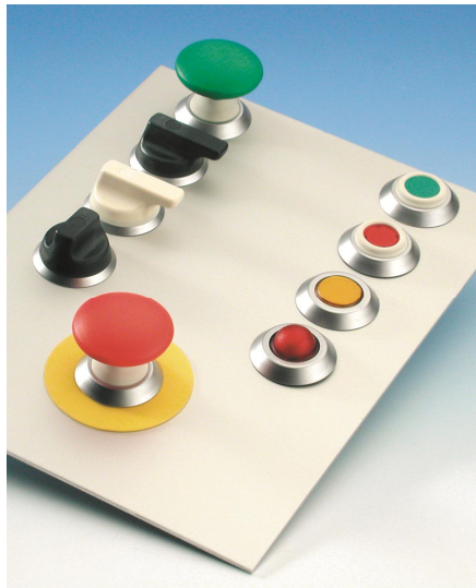
Fig. 42.39 Control panel with hygienic control and indicator devices. Seals should fill the gaps between the fixed and moving device parts, to avoid the ingress of product residues, lubricants and organic materials. A perfect, hermetic seal is also required to prevent the ingress of moisture, dust and dirt within the control panel. Adequate space should be provided between control and indicator devices for easy cleaning (courtesy of Elan-Schmersal).
