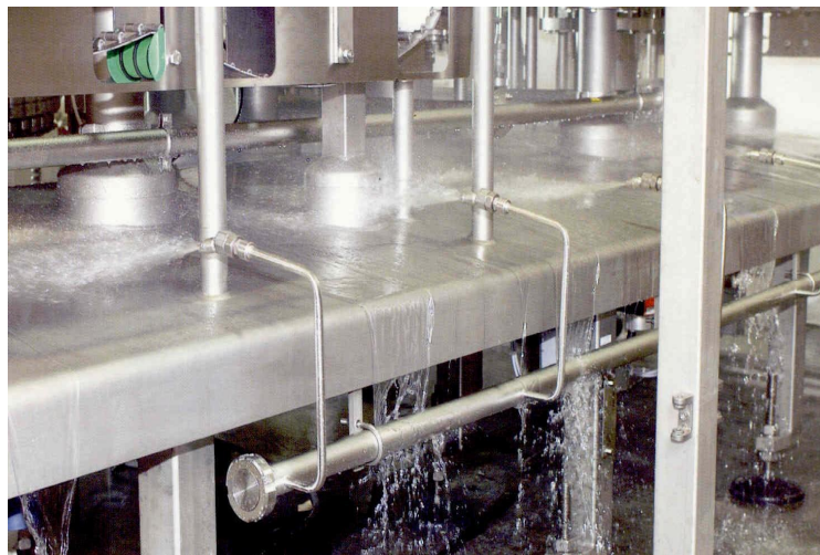
Fig. 42.2 All surfaces in the product zone are designed to be self-draining for liquid food, cleaning and disinfection solutions, and rinsing water (courtesy of Kronos)
