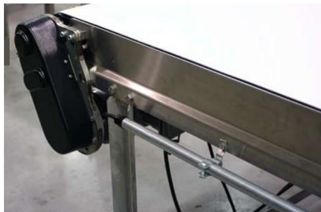
Fig. 42.33 Motors should be rather located below the line of the product flow. Both gears, chains and motors of belt drives must be covered to avoid any contamination of product. However, a chain guard (essential from an occupational safety point of view), when open, may provide a place where product may accumulate, allowing microbes to multiply to large numbers and so posing a contamination risk for the food product on the belt (courtesy of Dorner conveyors).
