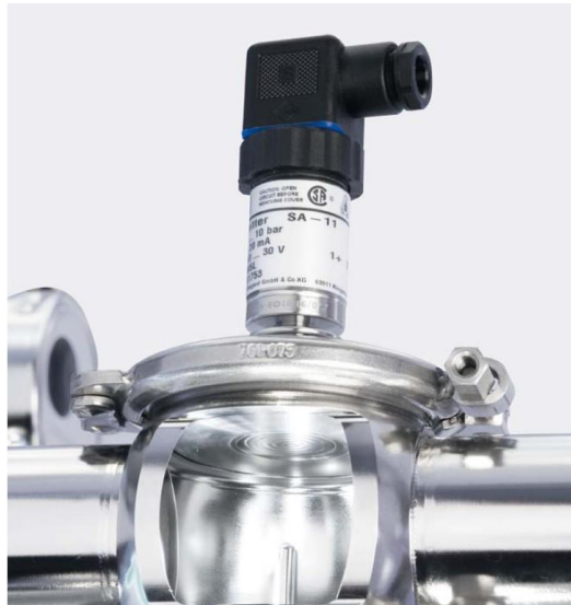
Fig. 42.52 Pressure transmitter with tubular membranes, having the same inner diameter as the adjacent pipeline, can be integrated into the process, installed by means of a clamp fitting in a standard spherical valve body welded into the piping. The stainless steel diaphragm is sealed by O-rings fitted into grooves such that there is no metal-to-metal joint on the product side. This way of mounting of a pressure transmitter provides a dead-space free, flush transition from the process line to the pressure transmitter (courtesy of WIKA).
